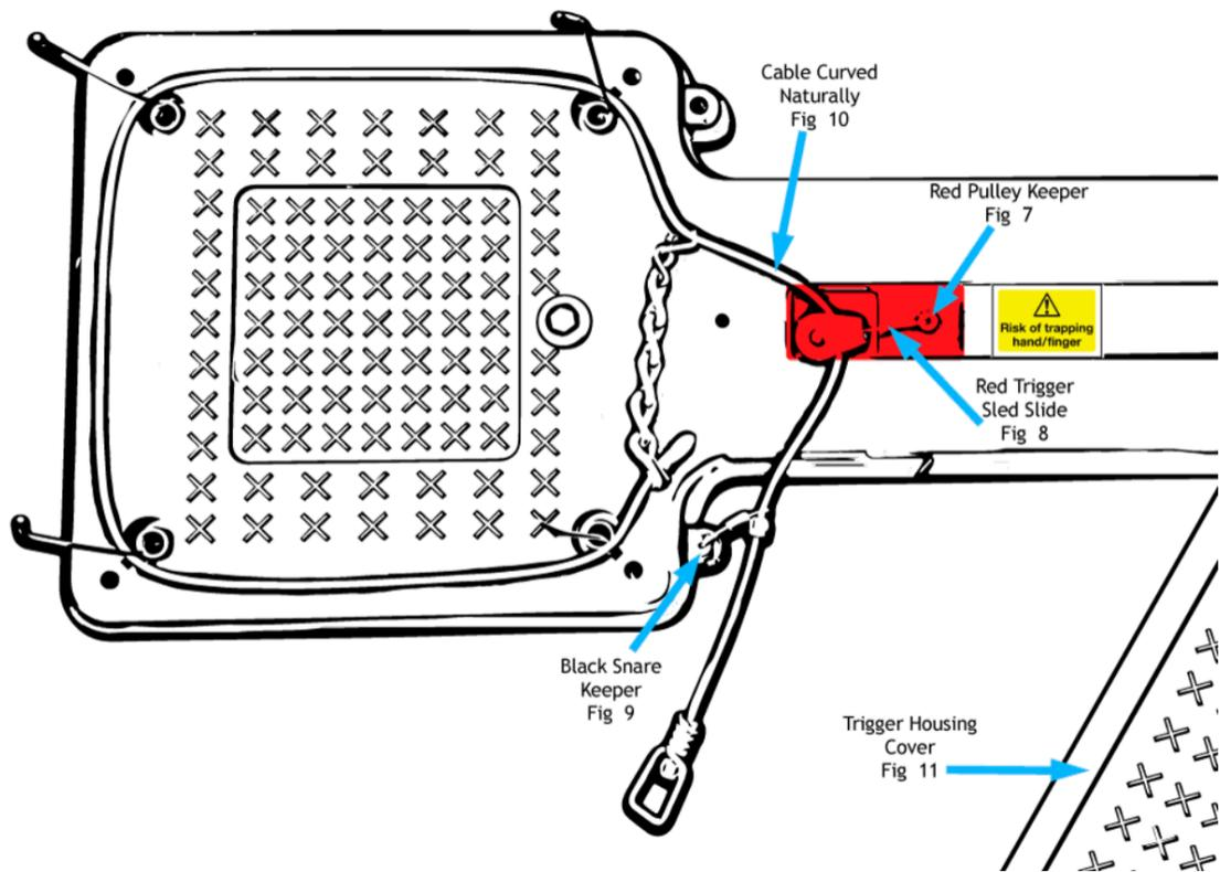
**f.** Place the trigger housing cover (**Fig 11**) on the neck of the unit. Place cover on top, completely covering the opening. **Make sure the writing on the cover is towards the pan**
